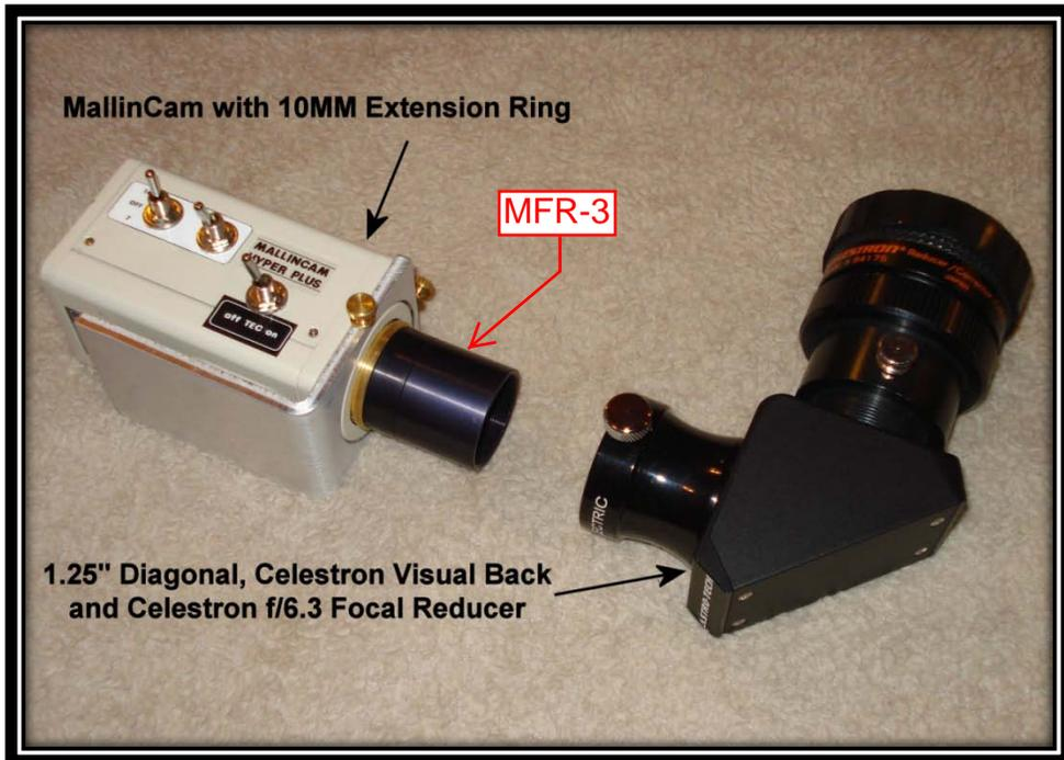
The assembly is screwed directly to the back of the SCT Optical Tube Assembly and the system speed will be f/4.
