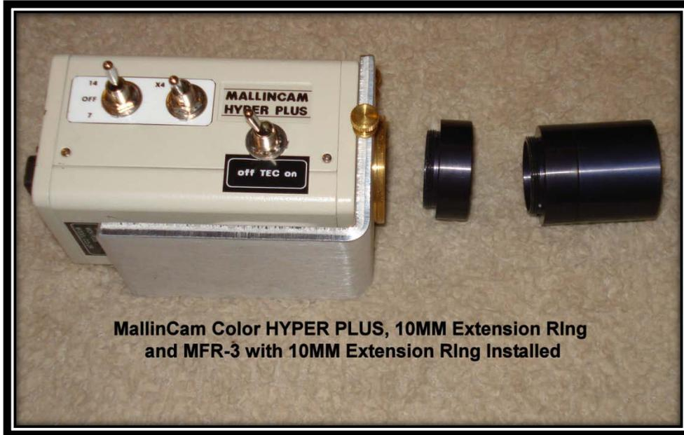
When two 10MM Extension Rings are inserted between the MallinCam and the MFR-3, the provided **FOCAL REDUCTION is 0.55.**
