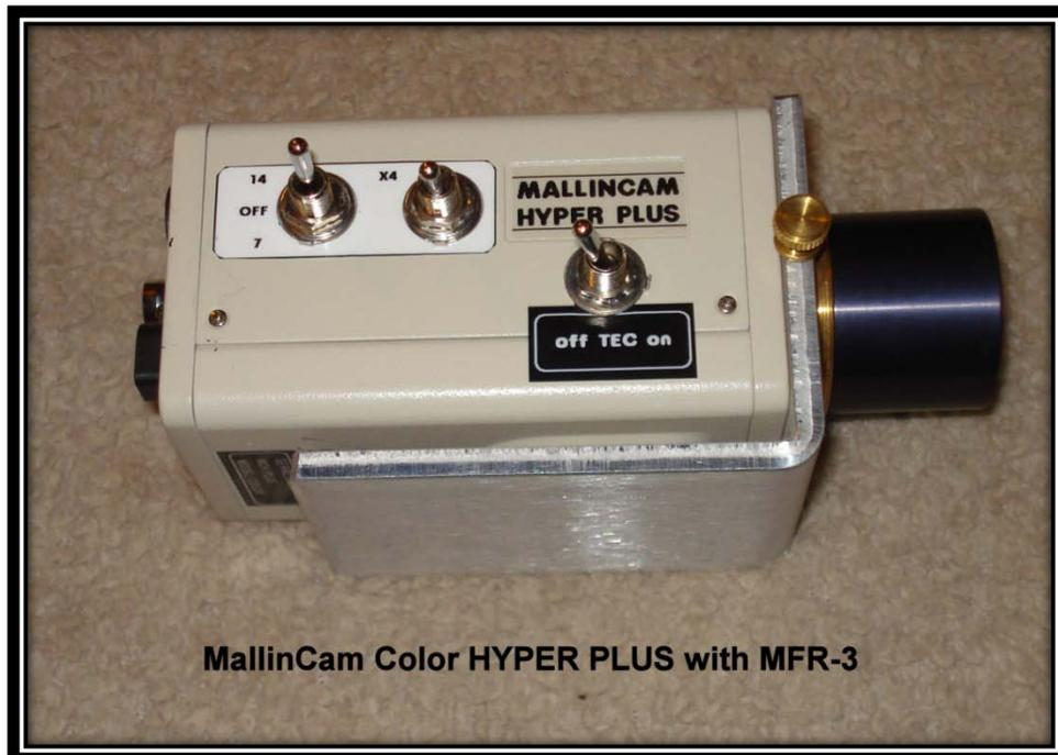
They look the same. The only way to tell them apart is to look into the front of the machined aluminum barrel to see if there is a lens present. Adding a 10MM Extension Ring between the MallinCam and the MFR-3 provides a **0.65 FOCAL REDUCTION**.
