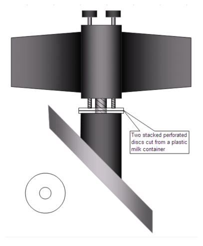
I would actually recommend the removal of the secondary at this stage anyway as you can perform a basic modification which will make step four a little easier. This is to add a 'milk carton' washer to the secondary stalk bearing surface (i.e between the three adjusters and the non mirror end of the stalk). Credit for this mod and the image above goes to our US friend Jason Khadder.
