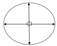
The method for this is to loosen the short side, holding both the vane (so it does not twist) and the nut and then tighten the long side sequentially until they are both the same length to the centre.
